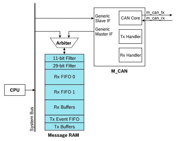
Figure 1: Integration of M\_CAN IP module into a system
